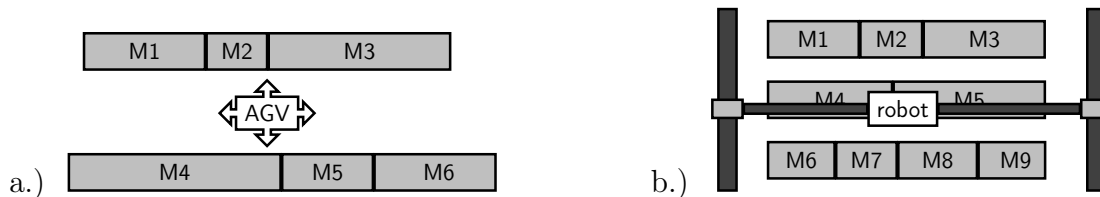
Figure 2.3: In a.) again an AGV moves pieces between the machines. For areas with limited space a gantry robot is required as displayed in b.).
